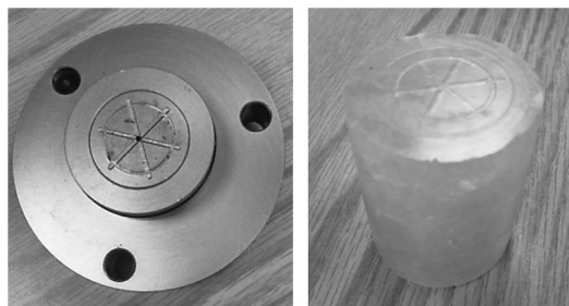
Figure 3. Print of pore pressure line pattern of (left) the buffer on the end surface of (right) the halite sample.
