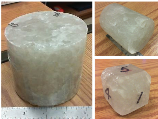
Figure 1. (left) Halite salt core and (right) samples made from it for ultrasonic velocity measurement and low-frequency measurement.
