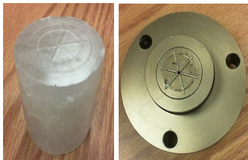
Figure 3: Dent of pore pressure line pattern on halite sample after measurement of 3 testing circles
