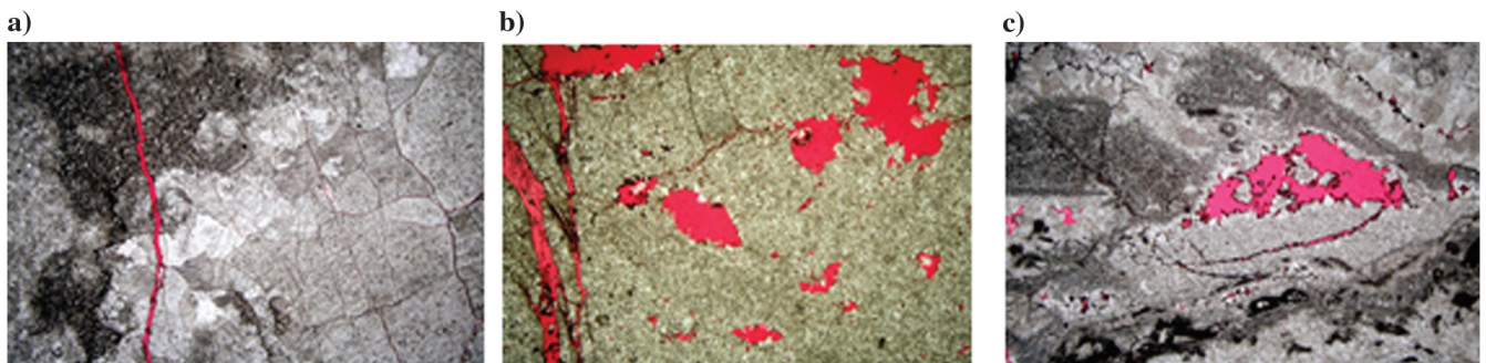
Figure 3. Core photos of reservoir rocks in the Yuanba gas field of Sichuan Basin, southwest China. Red parts represent pore space. (a) Fine-medium crystal dolomitic limestone with microfractures, (b) power crystal dolostone with vuggy pores and microfracture, and (c) power crystal dolostone with vuggy pores and microfractures.
